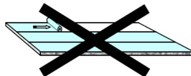
Roll out the foam down across the width of the room. ref 1027008 (1 roll = 1.6m width x 25m length = 40sqm) during 12 hours with no tension and without any storage on it.
