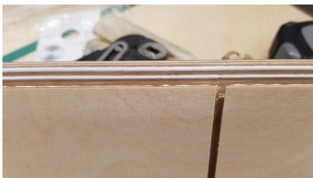
**Check that the glue is well dispatched on tongue and groove.**
