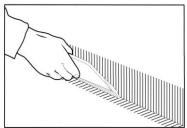
Using a straight edge and pencil, mark at a height of about 10 cm (approx. 4 in.) all walls where the flooring will be coved. Apply the adhesive on the walls up to the marked line, using a fine-notched trowel.
