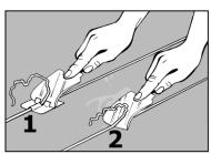
IMPORTANT: Both rough cut and fine trimming must be carried out while the welding rod is still lukewarm.
