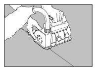
The sheets are hot welded. Do not weld until the adhesive has bonded completely, wait 24-48h. The joints are chamfered or grooved to about 3/4 of the thickness.
