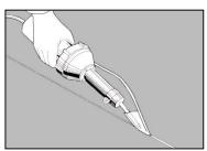
Weld with hot-air and Tarkett Speed Welding Nozzle.
