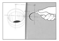
Around drain pipes, fold the sheet against the pipe and mark a line on the material where the centre of the pipe is. Cut an evenly round hole without notches along the cut, about 25 mm (about 1 in.) smaller than the diameter of the pipe.
