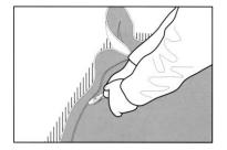
Avoid sharp creasing tools. When coving we highly recommend to use a Tarkett Hockey Stick or a Corner Roller to press the material firmly into the juncture between the floor and wall.
