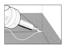
Use a hot-air gun for welding with thread at in-corners and out-corners. For a perfect job, the Swan Neck is required to effectively seal all seams nearest to the floor.
