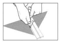
To glue the triangle-shaped piece more simply and securely, cut a groove on the back of the triangle with Corner Knife. The depth of the groove shall be no deeper than half of the sheet thickness.
