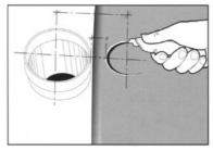
Around drain pipes, fold the sheet against the pipe and mark a line on the material where the center if the pipe is. Cut a hole about 25 mm (about 1 in.) smaller than the diameter of the pipe. As shown, cut the hole at the start of the fold. Heat the sheet vinyl and press it over the pipe. trim off excess material with a hook knife so that the break in the pipe wall is cleared.
