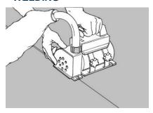
The sheets are heat welded. Do not weld until the adhesive has bonded completely. The joints are chamfered or grooved to about ¾ of the thickness using a hand grooving tool or machine prior to welding.
