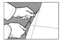
When the width of the room exceeds the sheet width (more than one piece has to be installed to cover the area), mark a line on the floor parallel to the longitudinal wall at a distance equivalent to 12 cm (about 41/2 in.) less than the sheet width. Mark the room's center on this line. On the bottom of each sheet, mark their center. The cross marks on the subfloor and sheets shall coincide at installation.
