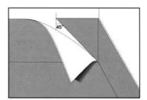
The corner seam shall be placed on one of the walls at a 45-degree angle.
