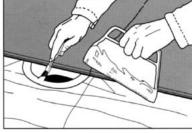
Fold back and loosen the sheets covering half of the floor area. Apply the adhesive on the subfloor with a fine-notched trowel. Use a soft brush around drains and hard-to-reach areas. Around and inside drains, please see drain manufacturers recommendation.
