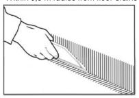
Using a straight edge and pencil, mark at a height of about 10 cm (approx. 4 in.) all walls where the flooring will be coved. Apply the adhesive on the walls up to the marked line, using a fine notched trowel. Spread some of the adhesive out onto the floor, as shown in the picture.
