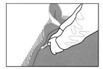
Use a Hockey Stick or Corner Roller to press the material firmly into the juncture between the floor and wall. In areas where one sheet is sufficient to cover the subfloor, the adhesive can be applied over the entire surface area before installing the sheet.
