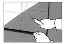
When fitting an out-corner, the sheet is folded against the corner and cut about 5 mm( ½ in.) from the floor. The guidelines in the picture show the corner on the sheet and the position of the cut at about a 45- degree angle. Then a diagonal cut is made as shown.
