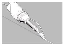
Weld with hot-air and Polystyl Speed Welding Nozzle. Carry out a test welding on a leftover piece before commencing work, to adjust speed and temperature.
