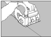
The sheets are hot welded. Do not weld until the adhesive has bonded completely, wait 24-48h. The joints are chamfered or grooved to about <sup>3</sup>/<sub>4</sub> of the thickness using a hand grooving tool or machine prior to welding.
