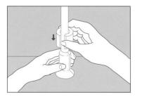
2) Prefabricated covers are applied according to the manufacturer's instructions. Seam sealer or sealing compound approved for this purpose, can be used for an extra tight fit around pipes.
