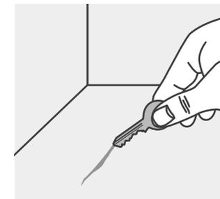
*When the subfloor is not hard enough, significant traffic or heavy load could damage screed/levelling compound and could cause visual/technical defects.*
