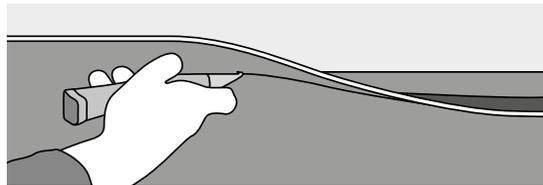
When gluing and pressing is done, excess of material close to walls and obstacles can be trimmed/flushed (freehand cut).
