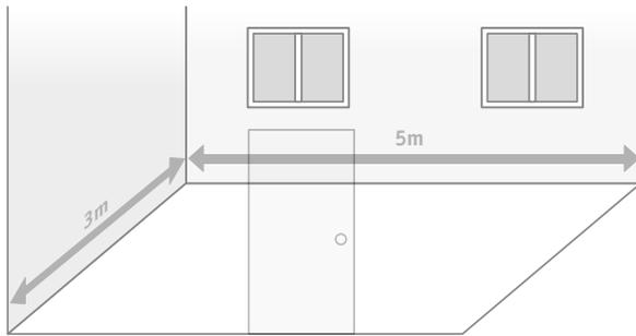
If the room is reasonably square, the sheets should run parallel to the incoming light. In long, narrow rooms it is best to install the sheets along the length of the room.
