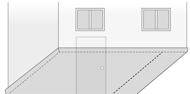
! Sections of flooring must be cut to the required lengths, plus an allowance of a few centimeters.
