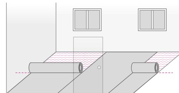
It's important to use the cork press when you gradually roll out the sheets onto the adhesive. In this way, you will avoid catching air under the sheets that may cause blisters later on.
