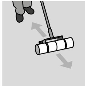
And then, use the heavy roller (mini 50kg) to ensure the final bonding.
