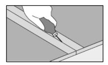
Apply the cold welding liquid by pressing the needle deeply into the seam. Fix a special masking tape, centered over the cut seam, then cut the masking tape with a rolling knife within the seam. Ensure you apply enough liquid along the entire joint. After 10 minutes the cold welding liquid on the masking tape should be dry and the masking tape is removed carefully backwards.
