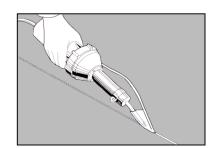
Weld with hot-air and Tarkett Speed Welding Nozzle. Carry out a test welding on a left-over piece before commencing work, to adjust speed and temperature.
