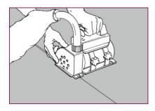
The tiles are heat welded. Do not weld until the adhesive has bonded completely. The joints are chamfered or grooved to about ¾ of the thickness using a hand grooving tool or machine prior to welding.
