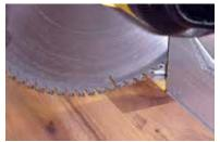
9. Use a carbide-tipped blade. Teeth of blade must cut into the decorative surface.
