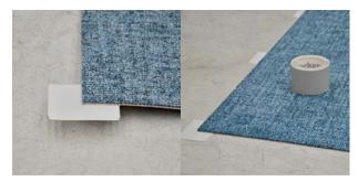
There are 324 units per roll. Each tape unit measures ca. 8 x 10 cm with notched perforations between each unit. The tape unit is centred at the corner of the tile as to engage the adjacent tile
