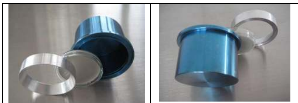
Figure 26 Outgassing test – cover ring
