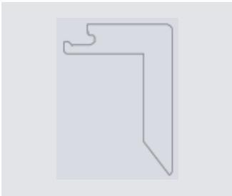
Stair nosing - Integrated 1 To be used with a floating floor installation to allow movements or to cover open steps. DIMENSIONS (LxWxHxT): 1950x52x72x14 FLOOR THICKNESS: 14 mm, 2-lock OAK, UNFINISHED: 8795250
