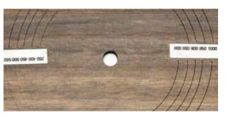
Scratch whitening is easier to see on dark surfaces than light ones. But even when we scratch-tested our darkest matte finish against the competitor's lighter wood grain pattern, Techtonic still performed better.
