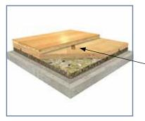
Targlue (PU mastic glue) and Targun have been specifically designed for the installation of Multiflex M. Applied with Targun, Targlue fixes the Tarflex subconstruction with the 14mm multi-layer.
