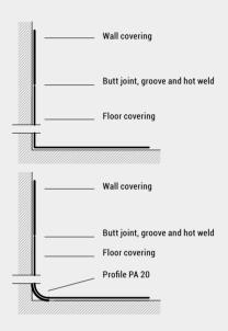
The sheets are hot welded. Do not weld until the adhesive has bonded completely, wait 24-48h. The joints are chamfered or grooved to about 34 of the thickness using a hand grooving tool. Weld with hot-air and Tarkett Speed Welding Nozzle, Welded seams must cool to room temperature before trimming in two steps, rough and fine trimming.
