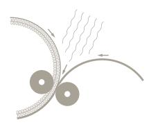
Heat and pressure "Powerbond" the wear layer to the closed-cell cushion, producing a floorcovering that is integral and inseparable.
