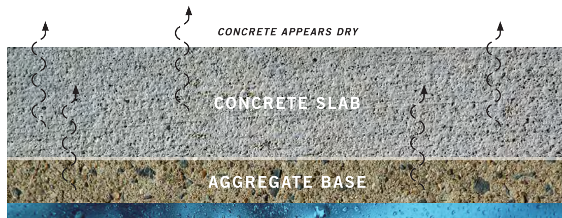
Fig F: VAPOR EMISSION GRADIENT CAUSES MOISTURE TO RISE
