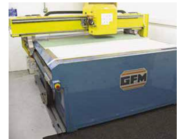
4 Cutting programs are transferred to our sonic cutting machines.
